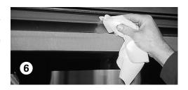
**Don't forget** to appropriately clean the cutting edges of the aluminium rail. This equally applies to the respective small contact face of the rear piece/front spoiler extensions within the TOP-RAIL rainwater gutter!
