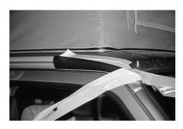
At the front, the front spoiler is fixed to the sheet with a masking tape: First, stick the masking tape onto the windscreen, then over the end of the spoiler and finally onto the driver's/passenger's window so that the front spoiler is properly placed and its peak pressed well onto the vehicle's sheet.
