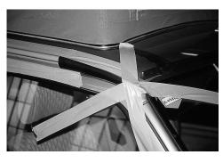
⚠ ATTENTION for every fixing with masking tape: Never follow the shape of the back part or the front spoiler! Put the masking tape onto the upper edge and fix it onto the sheet on a large scale. Thereby, the best strain is achieved.
