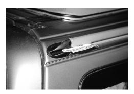
Please watch out that the piper entry is not blocked by adhesive remains and that the rear ending follows the piper rail of the aluminium profile without swelling. Hint: induct a piece of folded carton in matching diameter into the piper rail so that one part sticks in the aluminium profile and the other part in the back part and hereby appropriately widens the piper entry.
