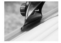
In order to calculate the permitted roof loading, you have to add up the dead weight of the entire roof load carrier and the weight of the loading.
