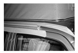
In order to acchieve a good sealing, the stripes have to be so thick that the adhesive protrudes a little above and beneath the profile when pushing TOP-RAIL against the surface.
