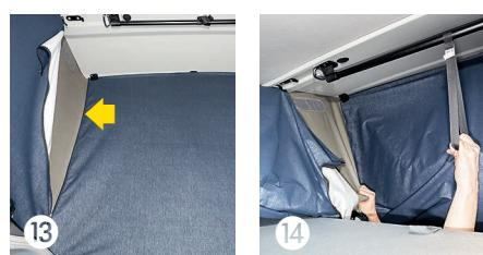
The self-drilling screws have to be screwed through the Pads into the lining. If you use a cordless screwdriver with torque, you have to adjust it on minimal moment of force and the screws mustn't screwed into completely – ATTENTION: Fasten the screws manually and carefully in the end to avoid overwinding!
