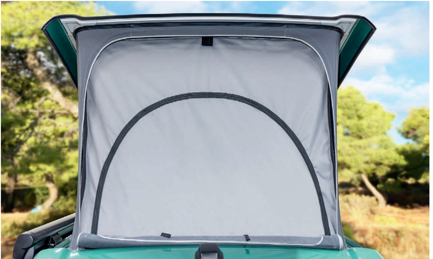
The front part as well as the FLYOUT of ISO-TOP MK VI have to be removed, when closing the pop-up roof.
