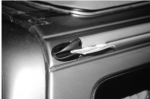
Please watch out that the piper entry is not blocked by adhesive remains and that the rear ending follows the piper rail of the aluminium profile without swelling. Hint: induct a piece of folded carton in matching diameter into the piper rail so that one part sticks in the aluminium profile and the other part in the back part and hereby appropriately widens the piper entry.
