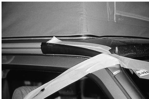
At the front, the front spoiler is fixed to the sheet with a masking tape: First, stick the masking tape onto the windscreen, then over the end of the spoiler and finally onto the driver’s/passenger’s window so that the front spoiler is properly placed and its peak pressed well onto the vehicle’s sheet.
