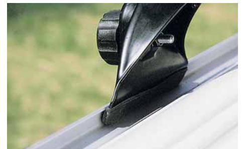
The supports of the carrier is fixed to the side and bottom of the rail, still allowing rain water to flow off easily.
