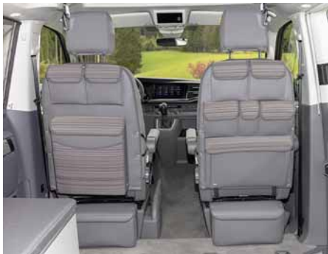
Utility with MULTIBOX for the left seat of the driver's cabin: insulation box + invisible rubbish bin + storage room. The MULTIBOX has the same quality as an insulation bag: its interior is lined with insulating and shock resistant material. It even offers enough space for 2 litre bottles. If you need a rubbish bin, simply insert a standard 20 litre rubbish bag with handles to the holders inside. Right side: the Utility for the passenger seat offers a lot of storage room. Design: "Mixed Dots/Leather Palladium". Made in Germany.
