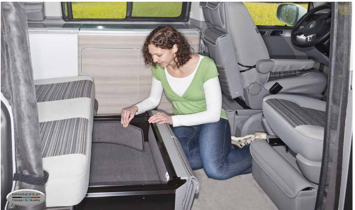
Noise damping mat and set T6.1/T6/T5 California: ideal to reduce noise inside the drawer beneath the bed (2-seater bench): deposited items do no longer "rattle" and are better protected. The awning crank can still be hooked in. The noise damping mat (floor) is simply placed into the drawer. The noise damping set (side parts) is attached with hook-and-loop fastener.
